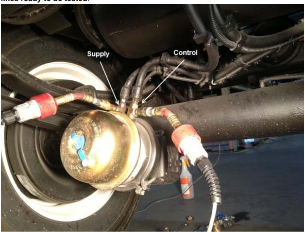
\*\*For the APPLY/RELEASE test and EMERGENCY PARK test any port on the LITE-CHECK HUB can be used.
